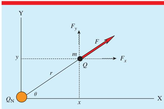
Figure 1. Alpha particle in field of nucleus.
