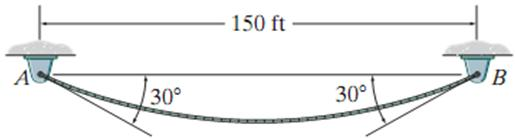
$$d := 75 \text{ ft} \quad \theta_M := -30 \text{ deg} \quad wo := 5 \frac{\text{lbf}}{\text{ft}} \quad \delta := \frac{d}{\text{m}}$$
